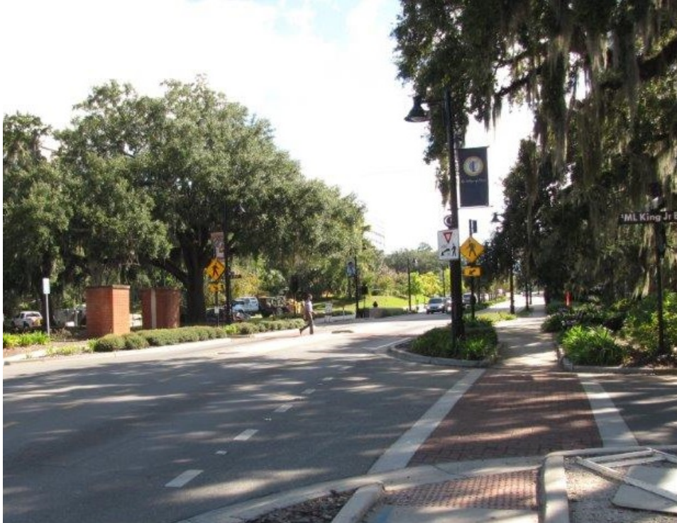
When walking across Gaines St, pedestrian marked crossings are not at corners, but rather midblock with pushbutton activated beacons. This shows a crossing from Burnette to Boulevard Park.
